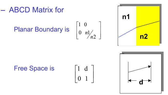
Equivalent Matrix of Cascaded Optical Components
